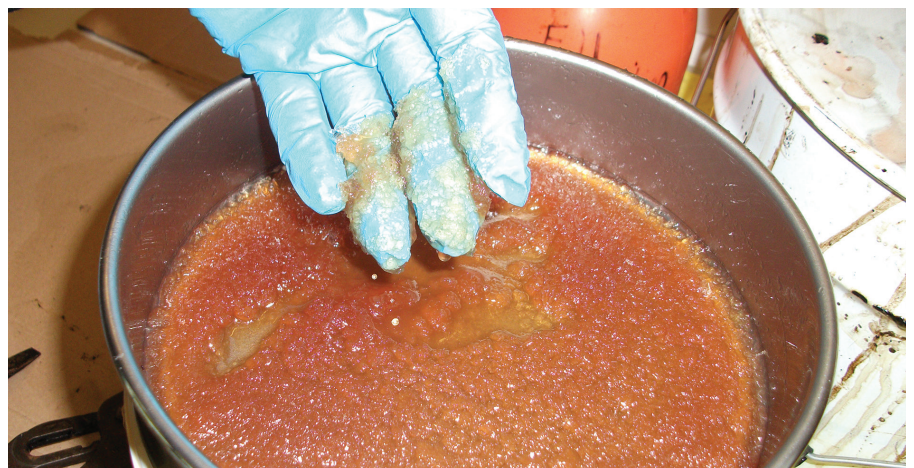
Fig. 33: Waxy precipitations in a fuel sample
