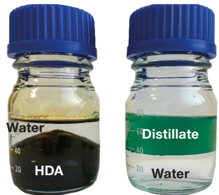
Fig. 46: The density of the HDA fuel is very high, even higher than water.
